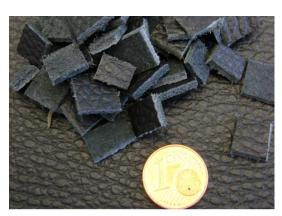
Fig. 1: Pre-punched leather chunks
