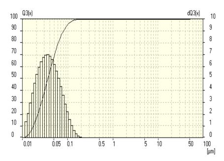
The depicted particle size distribution was measured with the FRITSCH Laser Particle Sizer ANALYSETTE 22 in consideration of the corresponding Mie parameters. With a comminution with a ball mill, a certain abrasion on the grinding bodies cannot be avoided. This occurring abrasion of the above measuring was deducted from the original.
