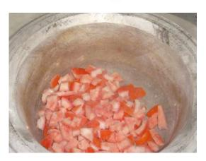
Fig. 2: Here the tomato pieces are floating in the liquid nitrogen inside the mortar bowl
