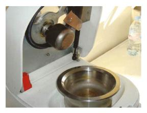
Fig. 1: PULVERISETTE 2 with Mortar bowl made of stainless steel
