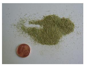
Fig. 6: Ground sample - 300 mg initial sample weight
