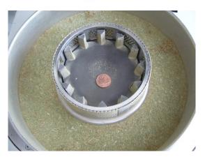
Fig. 4: Impact bar and 1 mm sieve
