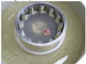
Fig. 5: Impact Bar and 0.0 8 mm sieve
